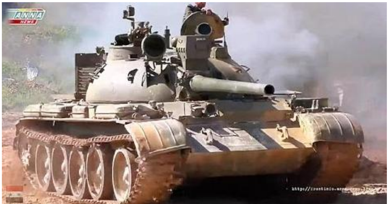
A T-55A with North Korean rangefinder and T-54-3 main gun in Syria
