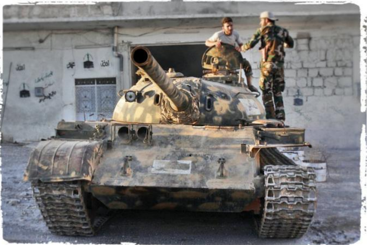
T-54-3 of the FSA 15 September 2013, Aleppo. This T-54-3 appears in a lot of photos and was captured by the rebels at the Aleppo Infantry Academy during December, 2012. Note the lack of a fume extractor on the barrel.
