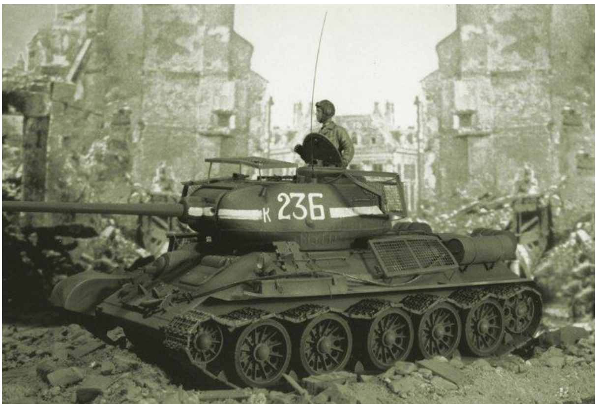
The old “radial-style” wheel on the T-34.
