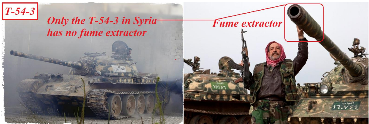
On the left is a T-54-3 in Aleppo. On the right is a tank with a fume extractor from the capture of the infantry academy in Aleppo City.
